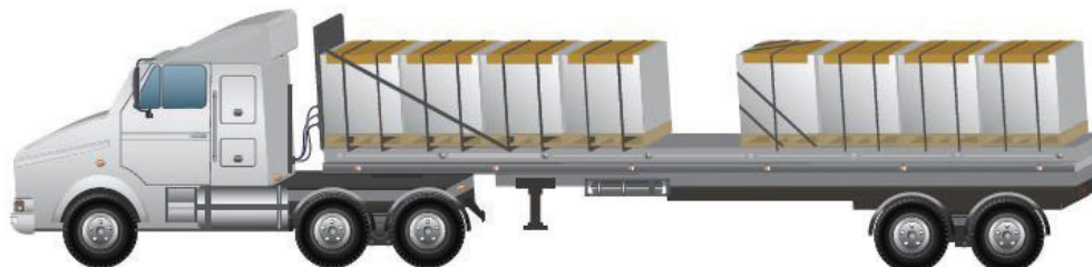
Left: Crossover webbing straps on unblocked load
